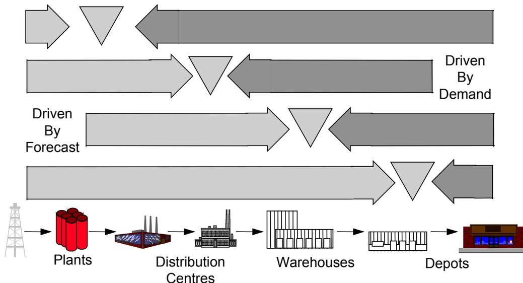
Postponement, or delayed configuration, is based on the principle of seeking to design products using common platforms, components or modules but where the final assembly or customisation does not take place until the final market destination and/or customer requirement is known.
